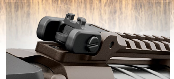
In the down position, the flip-up rear sights can be used in the standard rear notch/front blade configuration for fast target acquisition. In the up position, the rear sight is adjustable for windage and elevation and presents a sight picture similar to that of many modern sporting rifles.
