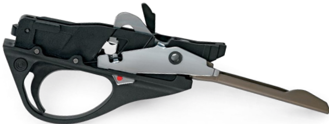
The Affinity 3.5's trigger group is easily removed for cleaning and maintenance by punching out a single pin.
