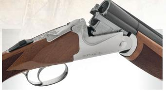
The Instinct SL receiver features a unique scalloped design and is fitted with automatic ejectors. The shotgun employs a locking bolt that emerges from the bottom of the standing breech to engage a recess machined into the barrel monobloc.
